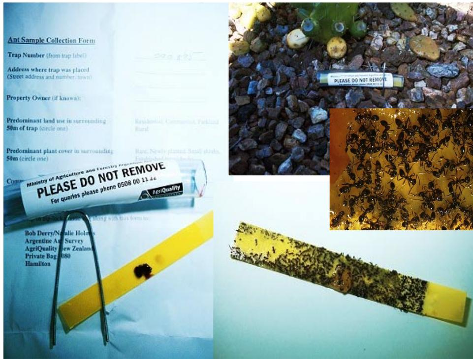
**Figure 1: Trap design and placement.**
